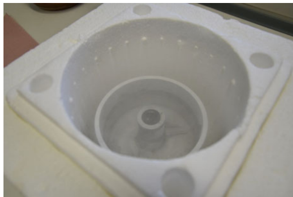
Fig. 3 A two compartment Al thermo-block filled with liquid nitrogen in outer and propane in inner compartment
